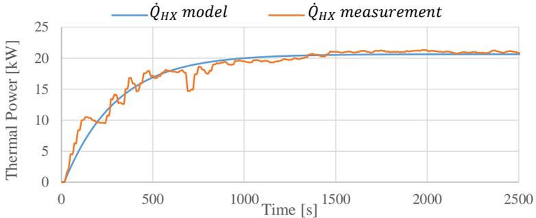
Fig. 7 Measured and modeled thermal power during a start-up phase
