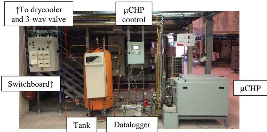
Fig. 2 Test facility (drycooler and 3-way valve are outside of the scope of the picture)
