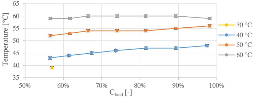
Fig. 6 Exhaust gas temperature versus inlet water temperature and load level
