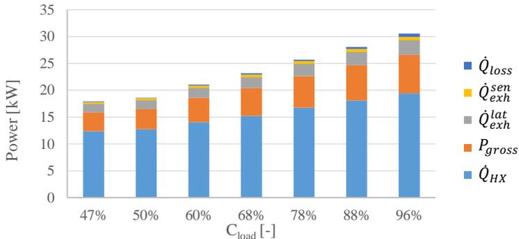
Fig. 5 Energy balance of the  $\mu$ CHP unit for different load levels and  $T_{cw,i} = 60$  °C, the total of each bar is gas consumption minus enthalpy of inlet air and gas (negligible)
