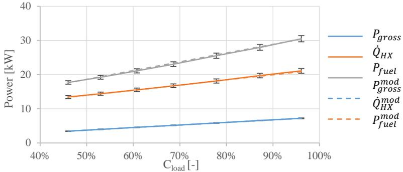
Fig. 3 Fuel consumption, electrical and thermal production for different load levels for 50 °C inlet water temperature
