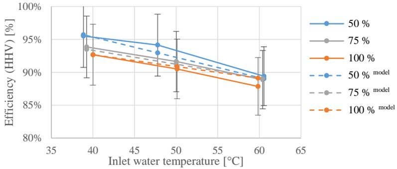
Fig. 4 Overall efficiency for 3 inlet water temperatures and 3 load levels (right caption)
