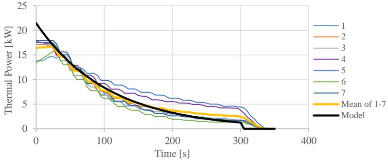
Fig. 1 Thermal power measured during 7 cooling phases of the  $\mu$ CHP, comparison to the mean of these series and the model
