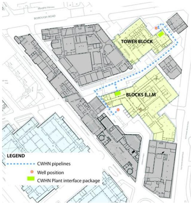
Figure 2: Proposed layout for CWHN demonstration.
