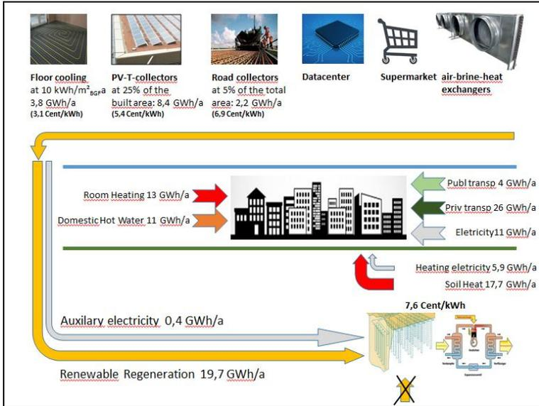
Fig. 2 Flow scheme of borehole based urban heat supply system
