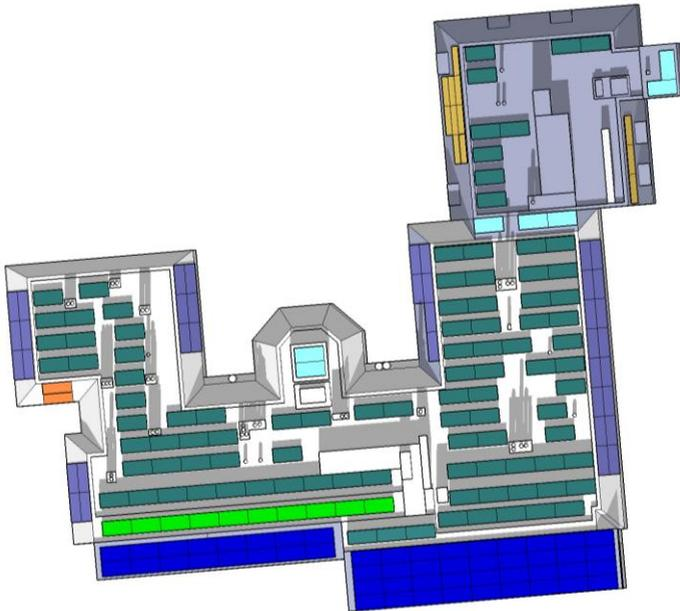
Fig. 5 Roof of the building equipped with the maximum amount of PV panels
