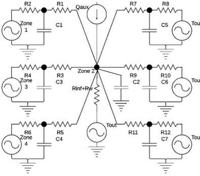
Fig. 3: DM schematic for main floor (Zone 2) (Interzonal resistances not shown)
