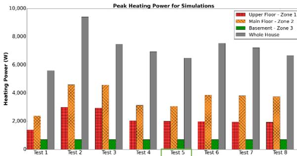
Fig. 10: Peak heating power simulation results for unoccupied basement tests
