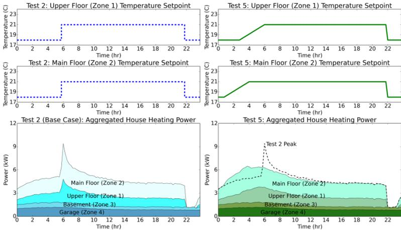
Fig. 12: Peak power results (unoccupied basement) for: (i) base case (Test 2) and (ii) advanced control strategy (Test 5)
