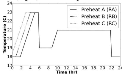
Fig. 9: Preheating (PH) temperature profiles with different start times
