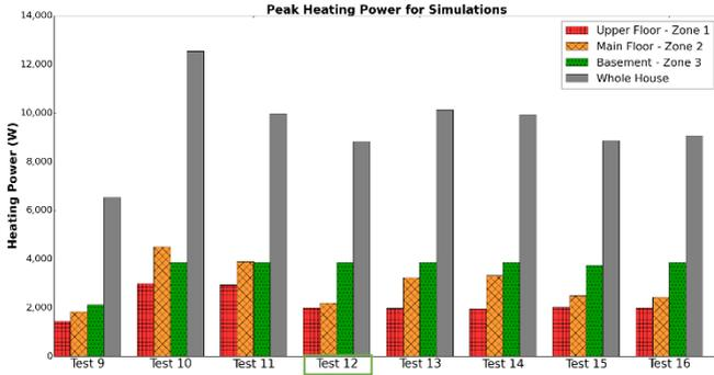
Fig. 11: Peak heating power simulation results for occupied basement tests
