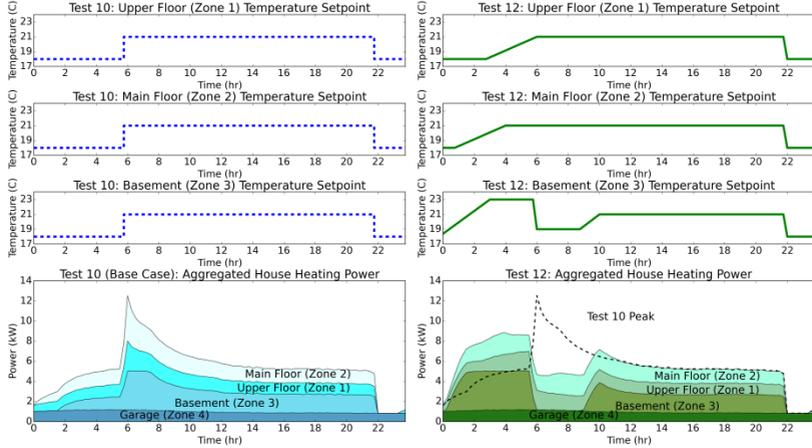
Fig. 13: Peak power results (occupied basement) for: (i) base case (Test 10) and (ii) advanced control strategy (Test 12)
