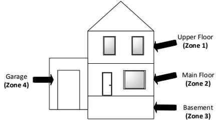
Fig. 2: Residential detached house modelled as 4 thermal zones
