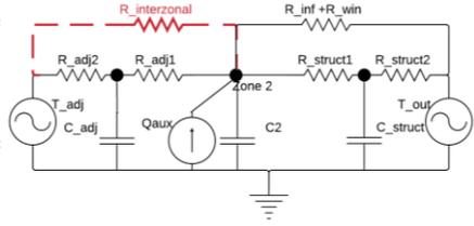
Fig. 4: SM1 (with red/bolded resistance) & SM2 schematics for main floor (Zone 2)
