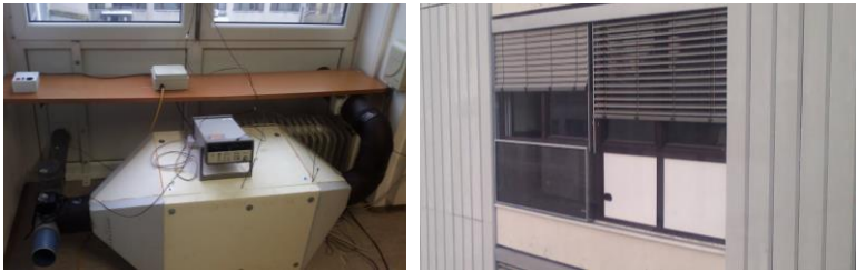
Figure 2: Experimental system: in room (left), solar air collector outside (right)
