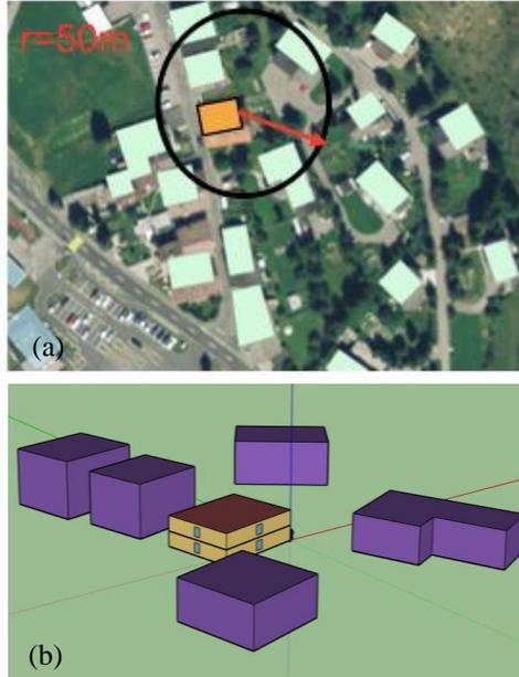
Figure 2. 2D Footprint of center Building  $B_i$  and neighbouring buildings  $B_{i+n}$  (a) and Resulting idf input file showing 3D thermal zones defined for center Building  $B_i$  and neighbouring buildings  $B_{i+n}$  in the neighbourhood  $N_i$  in an example district (b).
