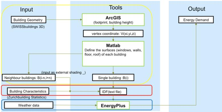
Figure 1. Workflow of the modelling and simulation process
