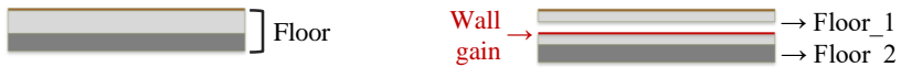
Figure 2: Conventional configuration of a floor in TRNSYS (left) and configuration with the added fictitious zone and the wall gain (right)
