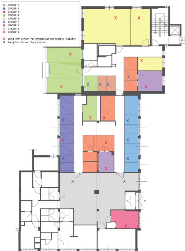
Figure 1 - Physiotherapy Center layout and locations of air temperature and relative humidity probes for long-term measurements.
