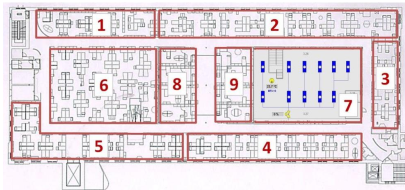
Fig. 2 The floor plan of 3 rd floor with marked sections of cooling beams (in section "7" the schema one of the regulatory branch is shown)
