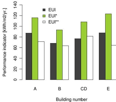
Fig. 2 Supplied annual energy use from the grid (except household elec.) to buildings A-E normalized with total heated floor area (EUI), with apartment floor area (EUI\*) and with envelope surface area (EUI\*\*).
