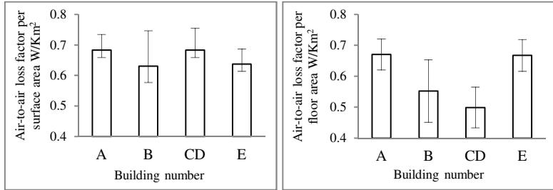
Fig.3 Regressed heat-loss factor ( $K_{tot}$ ) normalized against building envelope area above ground (left) and normalized against floor area (right). The error bars are 95% confidence intervals for the estimates.
