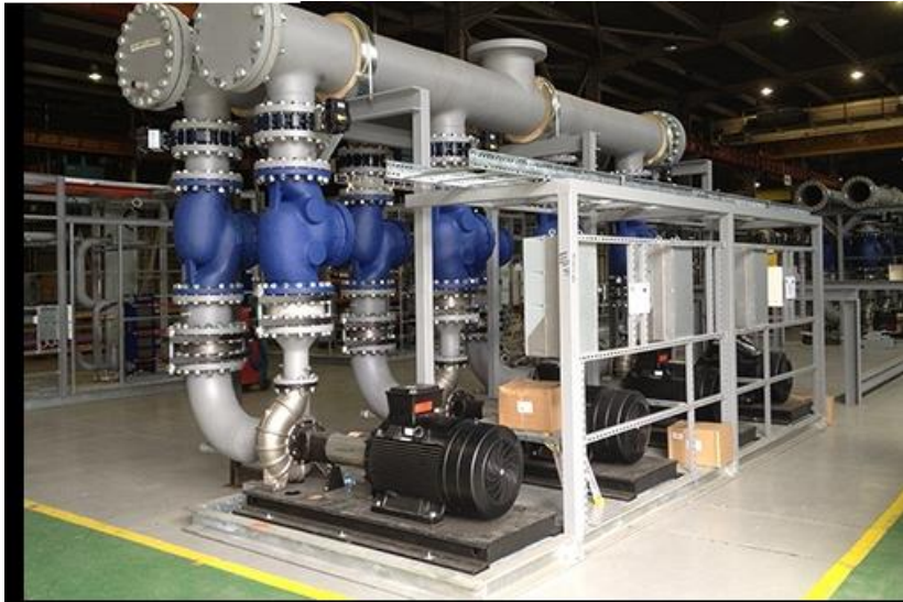
Fig. 2 Pump Skid Module for easy assembly offsite
