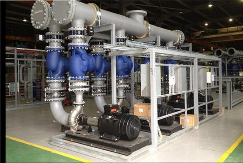
Fig. 2 Pump Skid Module for easy assembly offsite
