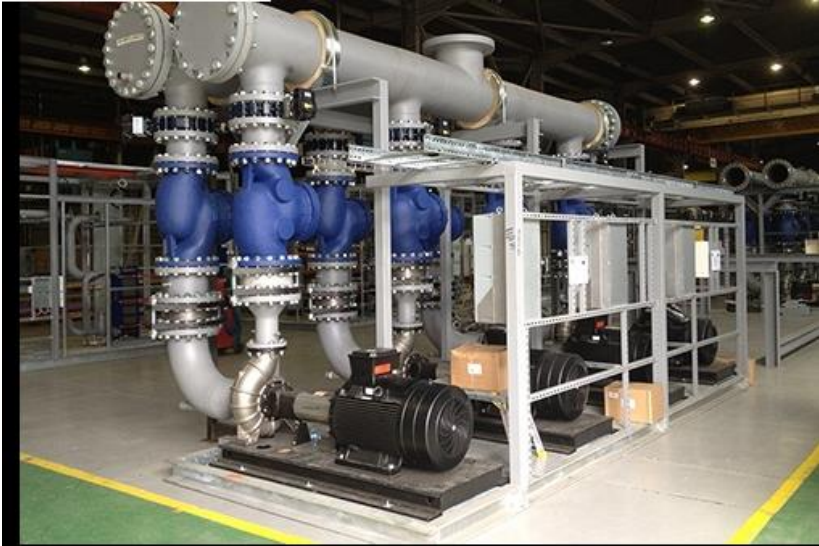
Fig. 2 Pump Skid Module for easy assembly offsite
