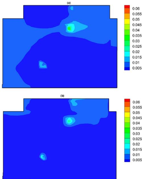
Fig.5 Comparison of CO<sub>2</sub> fraction distributions: (a) baseline case, (b) the optimal case
