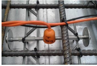
Fig 5 Example of smart-embedded building sensor
