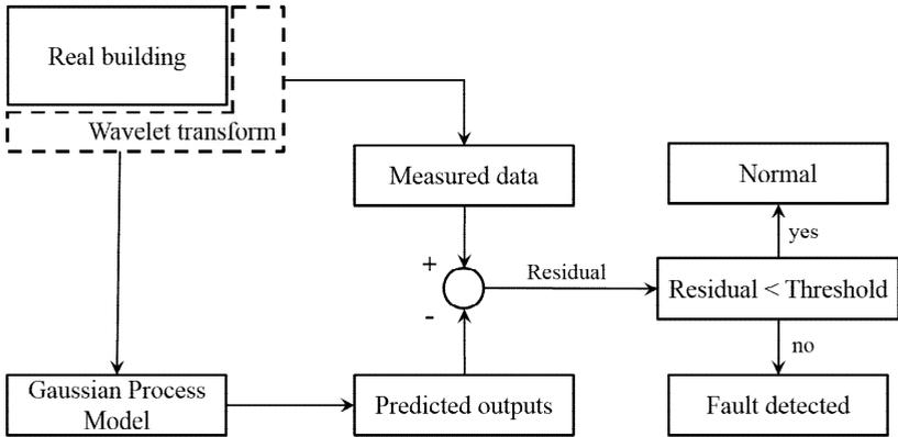
Fig. 3 Approach for sensor filtering and fault detection
