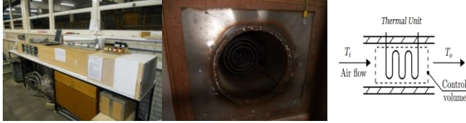
Fig. 1. The TU test-bed and schematic description of the TU
