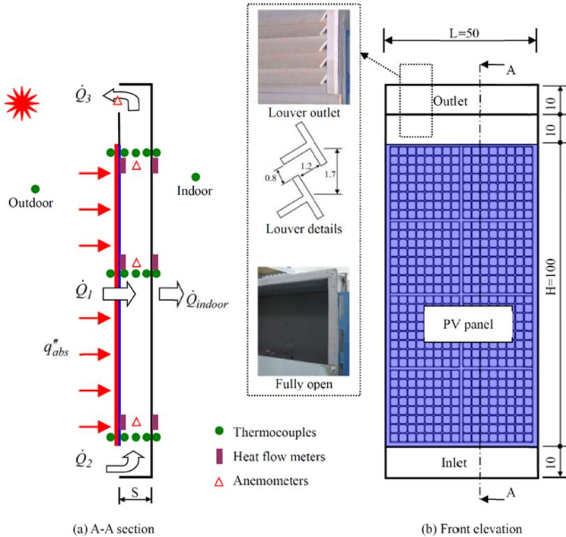
Fig.1 The tested ventilated BIPV curtain walls and measurement locations (unit: cm)
