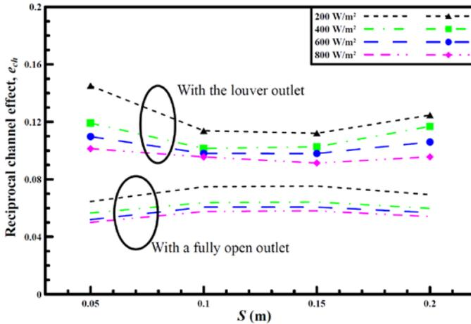
Fig. 2 Variations of the reciprocal channel effects ( $e_{ch}$ ) with the channel widths ( $S$ ) for various solar heating conditions and outlet configurations.
