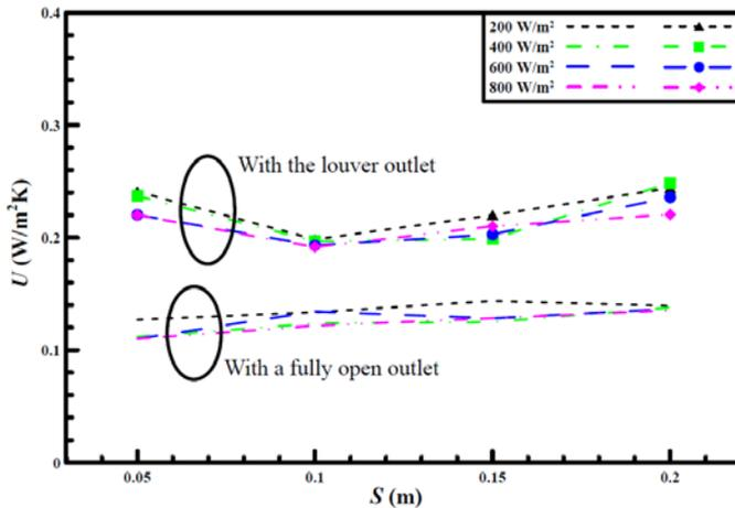
Fig. 3 Variations of the overall heat transfer coefficient ( $U$ ) with the channel widths ( $S$ ) for various solar heating conditions and outlet configurations.
