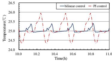
Fig. 6 Control performance of the space temperature on simulation platform
