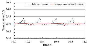
Fig. 7 Control performance of the space temperature with water tank
