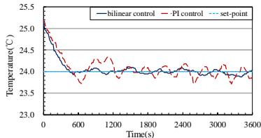
Fig. 9 Control performance of the space temperature on the experimental platform
