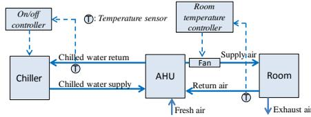
Fig. 1 Schematic diagram of the chiller integrated VAV A/C system
