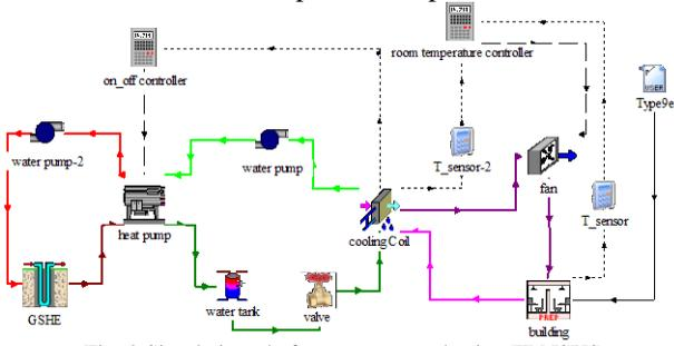
Fig. 2 Simulation platform constructed using TRNSYS
