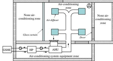
Fig. 3 Layout of the GSHP integrated AC system
