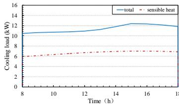
Fig. 5 Load condition of the room during the system operation period
