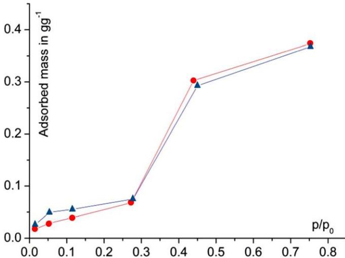
Figure 6 Equilibrium water desorption isobars of a representative mp-AF@Al coating after 1500 (●) and 4500 cycles (▲) [7].
