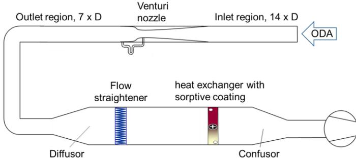
Figure 8 Schematic test set up for capacity tests of sorption material
