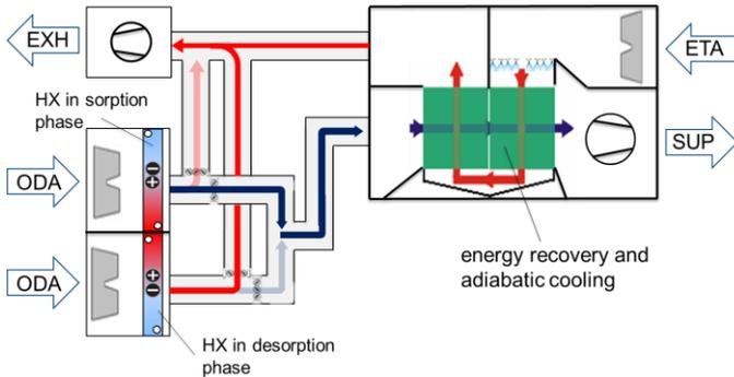
Figure 4 Concept of Thermal Driven Cooling
