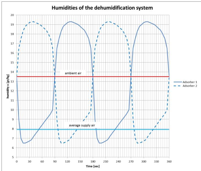
Figure 10 Switch over process for continuous operation
