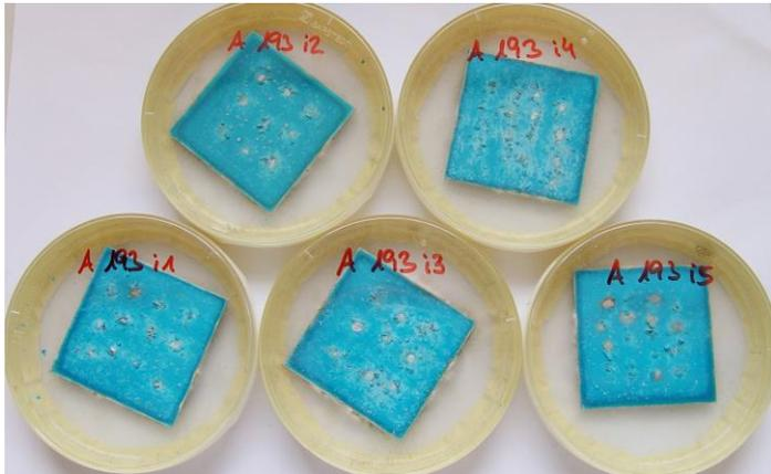
Figure 7 Material samples after 4 weeks of breeding at 24 °C and 95 % rel. humidity
