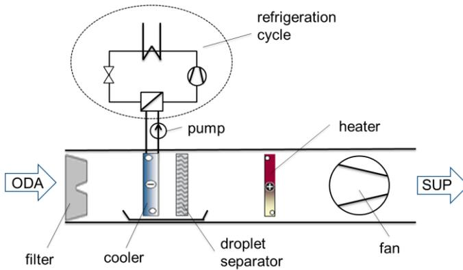
Fig. 2 Air handling unit for air conditioning and refrigeration cycle
