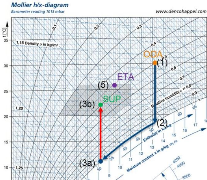
Figure 3 Cooling and dehumidification process (compression cooling)
