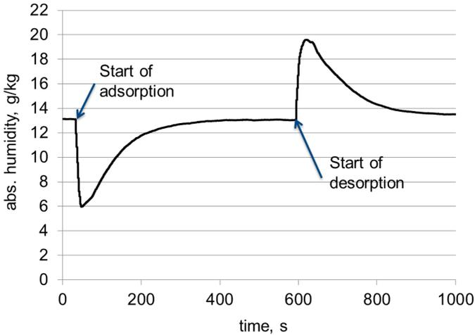
Figure 9 Absolute humidity for one test cycles (adsorption & desorption) with an air velocity of  $v = 1.4$  m/s
