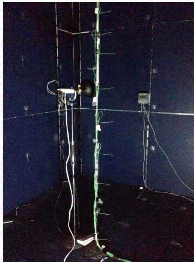
Fig. 4 Black globe, hot-wire anemometer and vertical temperature sensors
