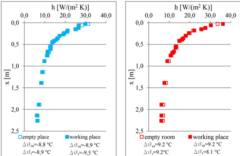
Fig. 9: Comparison of local CHTC for mixed convection at  $v_{sa} = 4\text{ m/s}$  on cooled (left) and on the heated TARS (right) for empty room and for the room with working place
