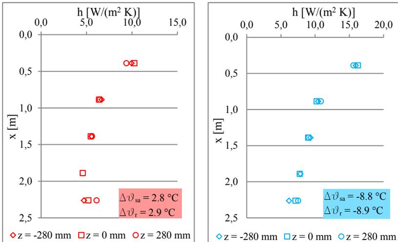
Fig. 3: Comparison of local CHTC for mixed convection at different widths on heated TARS at  $v_{sa} = 2$  m/s (left) and on cooled TARS at  $v_{sa} = 4$  m/s (right)
