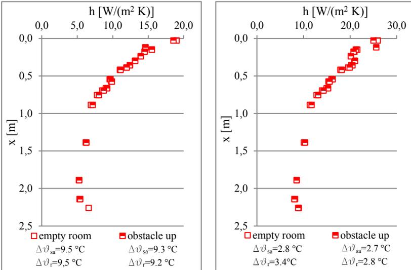
Fig. 6: Comparison of local CHTC for mixed convection on heated TARS at  $v_{sa} = 2$  m/s (left) and  $v_{sa} = 4$  m/s (right) for empty room and for the room with flow obstacle below of the ceiling
