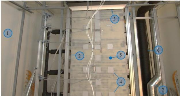
Fig. 1 Vertical TARS during installation of experimental setup into the thermostatic chamber: 1 – thermostatic chamber's wall, 2 – vertical TARS, 3 – slot diffuser, 4 – heat flux sensors with integrated temperature sensors, 5 – polypropylene, 6 – supply air duct, 7 – exhaust air duct
