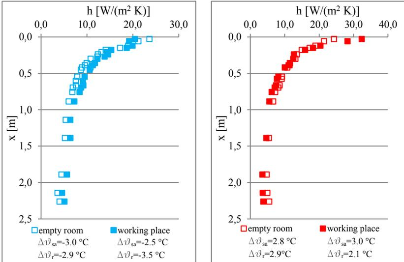
Fig. 8: Comparison of local CHTC for mixed convection at  $v_{sa} = 2\text{ m/s}$  on cooled (left) and on heated TARS (right) for empty room and for the room with the working place
