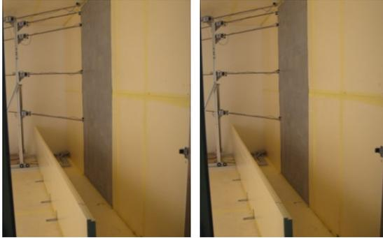
Fig. 4: Flow obstacles parallel to TARS alternately on floor and below of the ceiling
