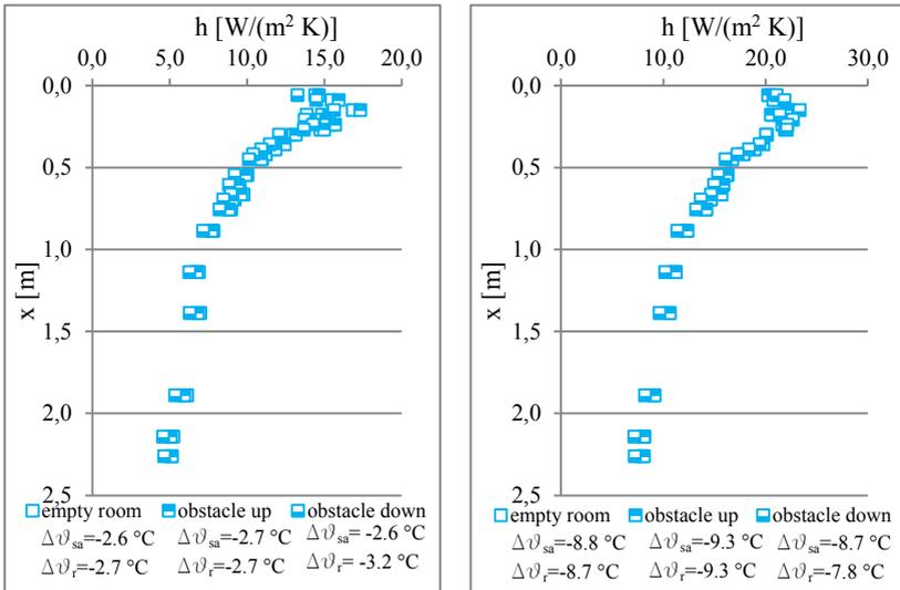
Fig. 5: Comparison of local CHTC for mixed convection on cooled TARS at  $v_{sa} = 2$  m/s (left) and  $v_{sa} = 4$  m/s (right) for empty room and for the room alternately with flow obstacle on floor and below of the ceiling
