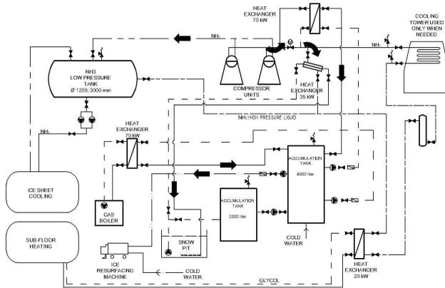
Fig. 3 Connection Scheme in the Ice Arena in Vlašim
