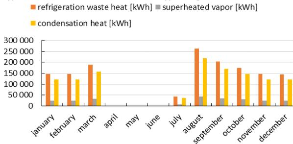
Fig. 4 Refrigeration Heat Dissolution during One Year
