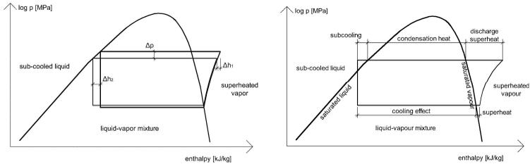
Fig.1 Compressor Cooling Cycle in the Pressure-Enthalpy Diagram
