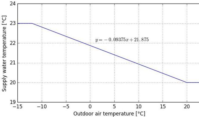
Fig. 2 Supply water temperature vs. outdoor air temperature
