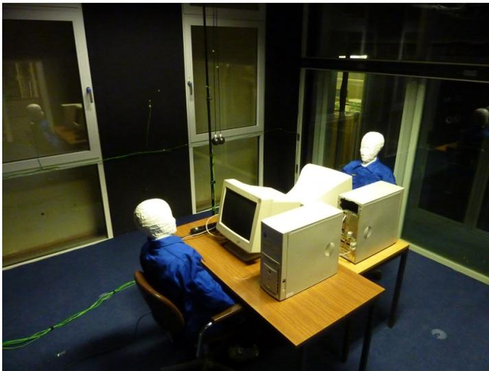
Fig. 3 Test chamber with two office working places and globe thermometers
