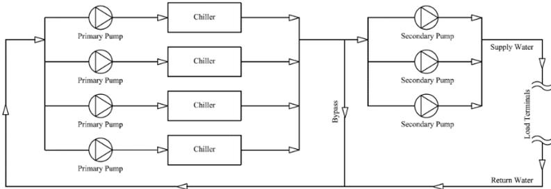
Fig. 1 A schematic diagram for the primary-secondary configuration
