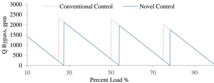
Fig. 2 The effect on the volume flow rate in the bypass with changing the primary pumps operation set points
