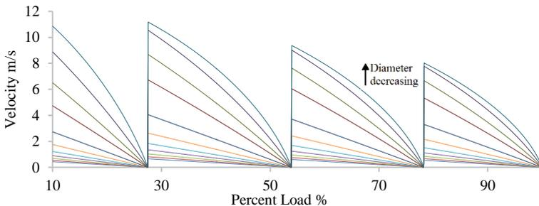
Fig. 4 The effect on the bypass average flow velocity in variable pipe diameters
