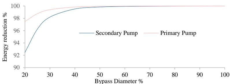
Fig. 5 The effect of changing the bypass diameter on the pumping power
