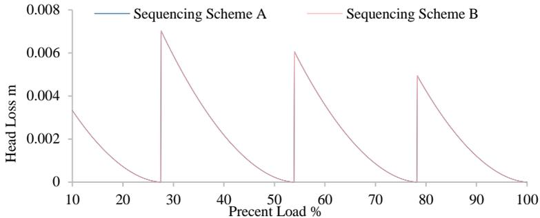
Fig. 3 The pressure drop inside the bypass for different secondary pumps sequencing strategies
