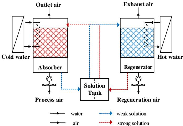
Fig. 1 Schematic diagram of liquid desiccant dehumidifier
