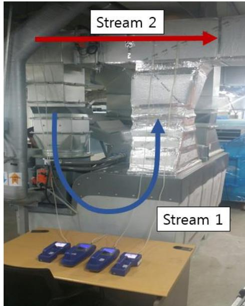
Fig. 2 Liquid desiccant dehumidifier
