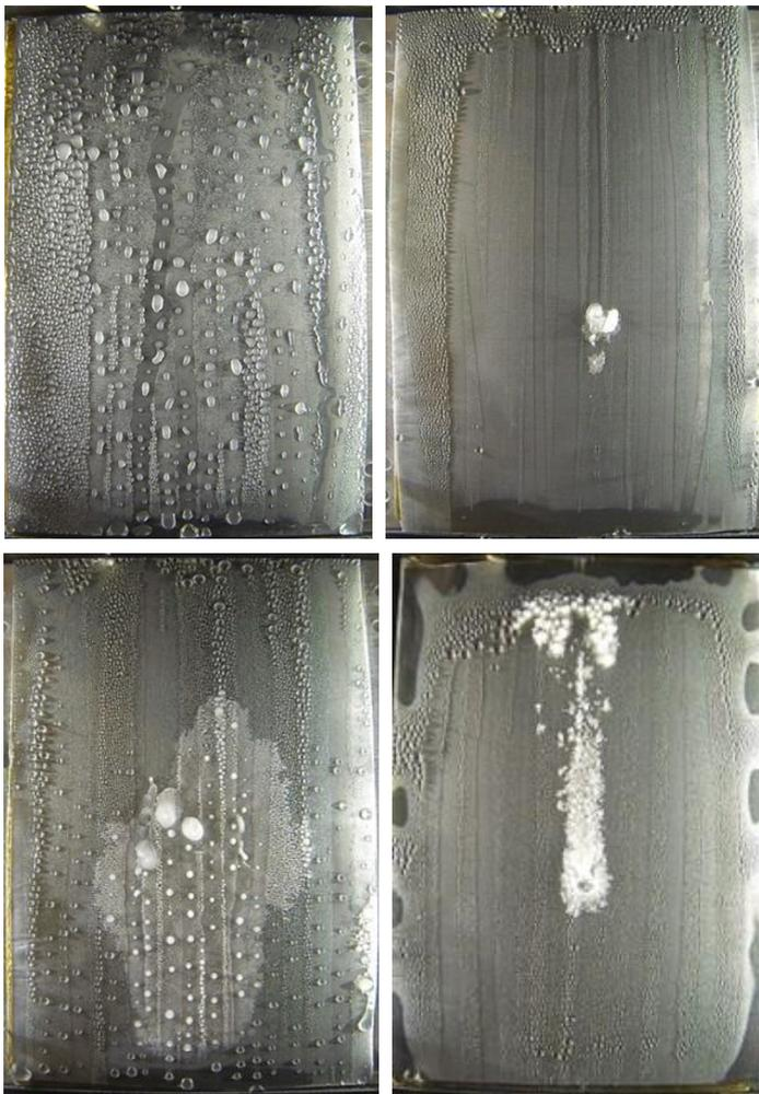
Frost spreading on wet surfaces at  $-4^{\circ}\text{C}$ . Freezing was initiated in the center of each of the four plates at  $t = 0$ . Opaque drops/areas (after 1 min) or white areas (after 20–45 min) indicate frozen areas.
