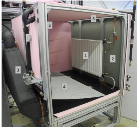
Figure 3: Setup of the test bench cabins: 1) radiator, 2) tempered walls, 3) supply air box, 4) slowed air inlet, 5) air outlet.
