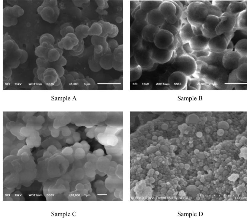
Fig. 2 Morphology of MicroPCMs synthesized by different types of emulsifier
