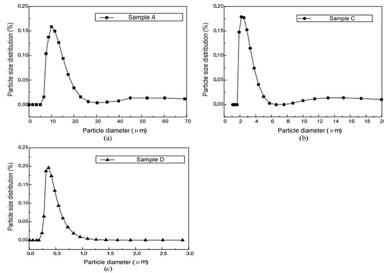
Fig. 4 Particle size distribution of sample A, C and D
