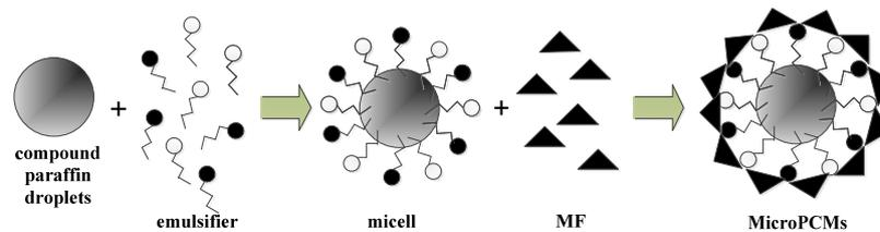
Fig. 1 The experimental principle of MicroPCMs prepared by in-situ polymerization
