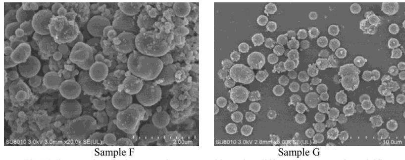
Fig.5. Micrographs of microcapsules prepared by using different contents of emulsifier
