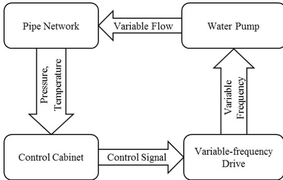
Fig. 1 Schematic diagram of variable flow system
