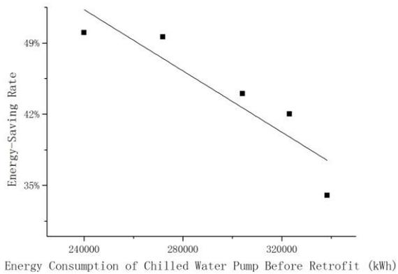
Fig. 4 Correlation between energy-saving rate and energy consumption of chilled water pumps before reconstruction
