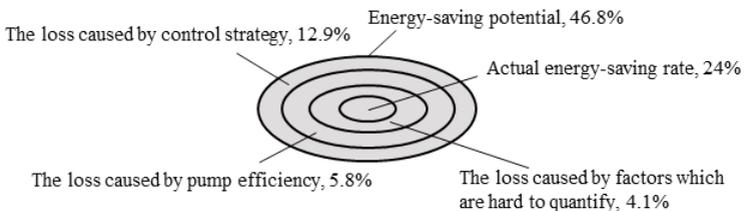
Fig. 6 Effect of factors on energy saving for No.12 building
