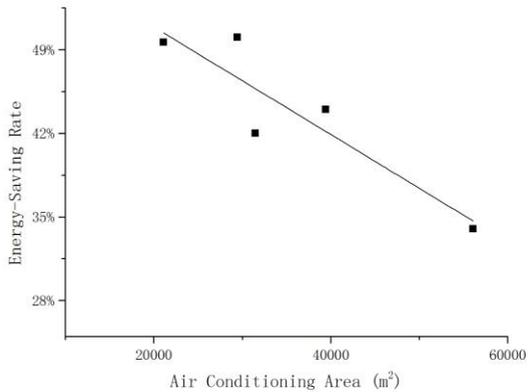
Fig. 3 Correlation between energy-saving rate and air-conditioning area
