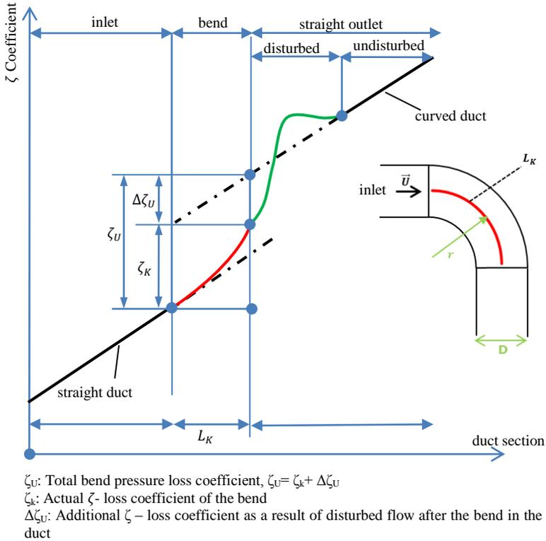
Fig. 2 Description of the pressure loss coefficient for a fitting
