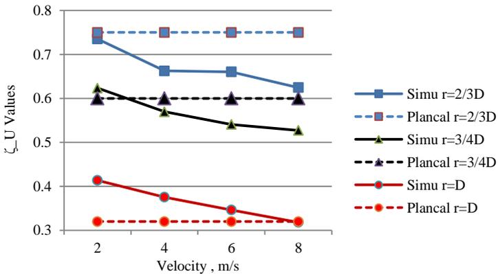
Fig. 5 Comparison of the  $\zeta_U$  values between the simulations and Plancal for the circular shape and the different radiuses of curvatures and shapes in dependence on the velocity.
