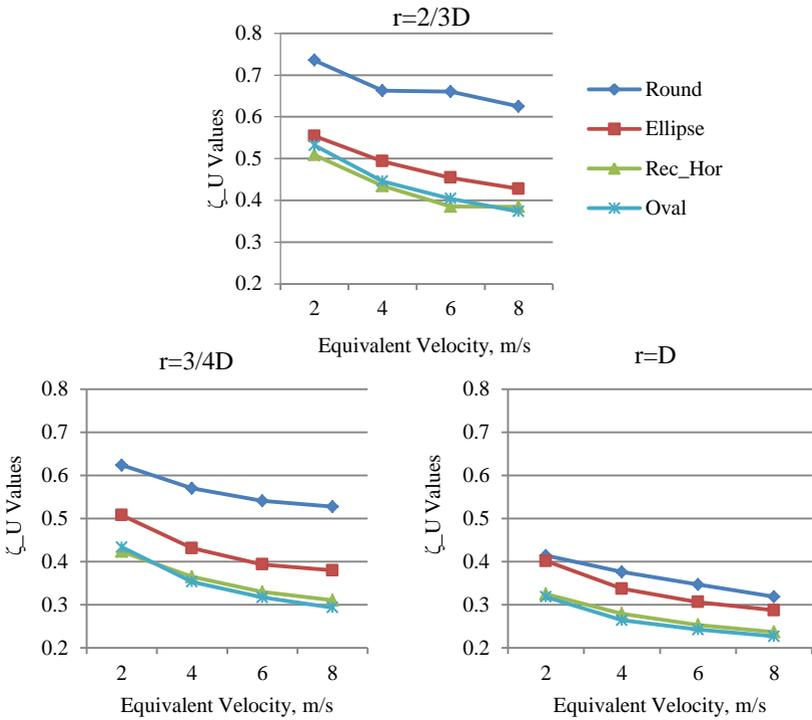
Fig. 4  $\zeta_U$  values for the different curvature radiuses and shapes in dependence on the velocity
