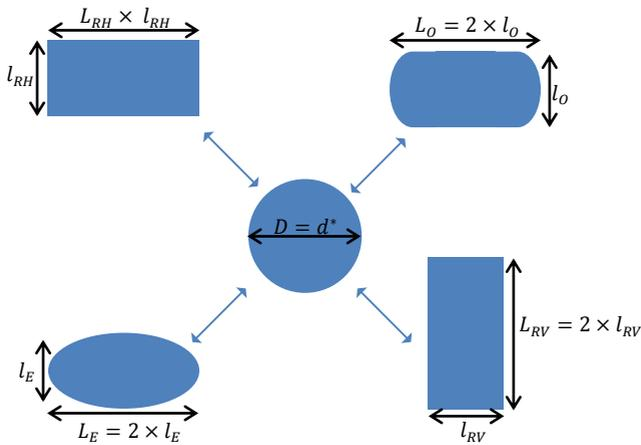
Fig. 3 Details about the different shape dimensions
