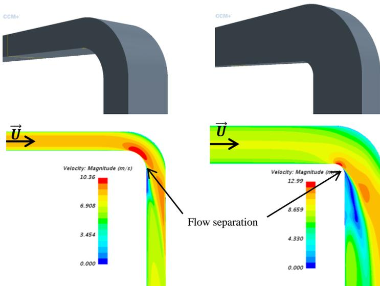
Fig. 7 Flow separation for bends of the rectangular vertical and horizontal shapes, equivalent velocity is 8 m/s and  $r = D$
