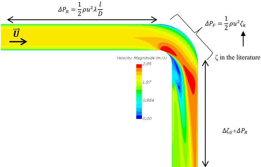
Fig. 1 Description of the pressure drop in a HVAC network
