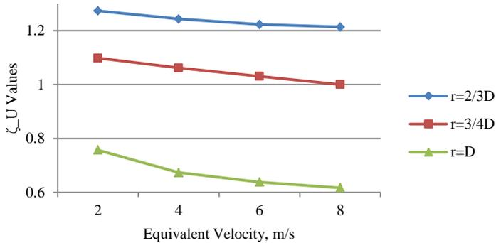
Fig. 6  $\zeta_U$  Values for the rectangular vertical shape for the different radius curvatures in dependence on the velocity
