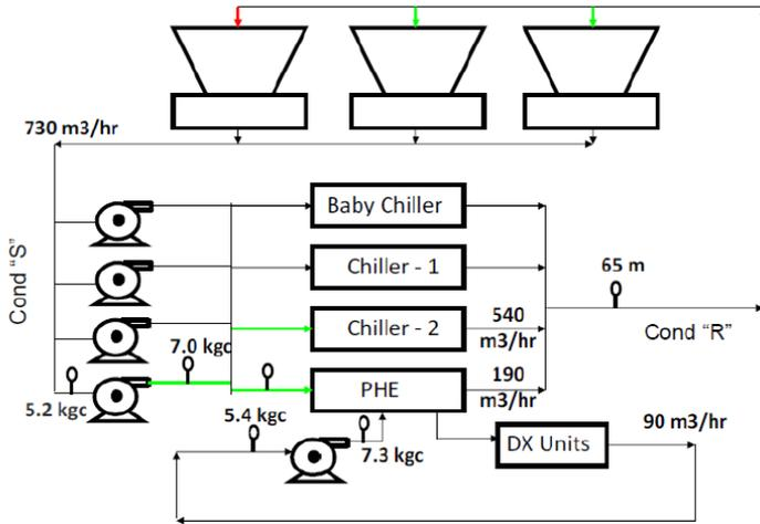
Fig. 5. Schematic diagram for cooling tower, pumps, chiller and PHE
