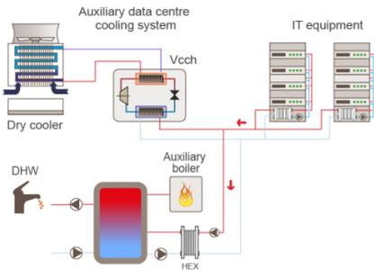
Fig. 4 Thermal scheme of a liquid cooled data centre connected to a residential building DHW system.
