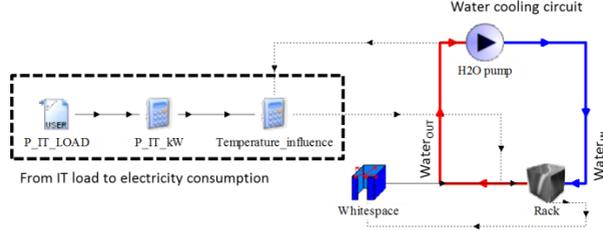
Fig. 1 Scheme diagram of the TRNSYS model for the liquid cooled data centre.
