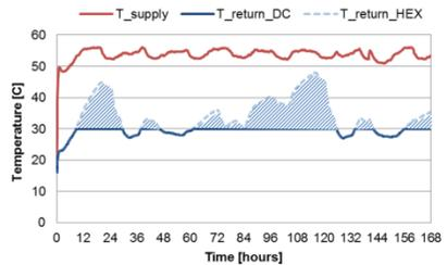
Fig. 7 Water temperature profiles in the data centre for 1 week of January
