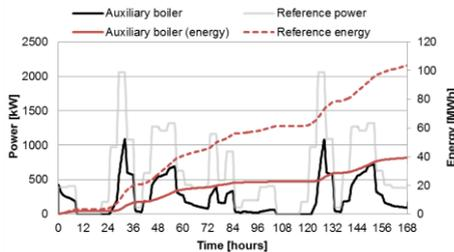
Fig. 8. Heater power and energy consumption for the system and reference system during a week.
