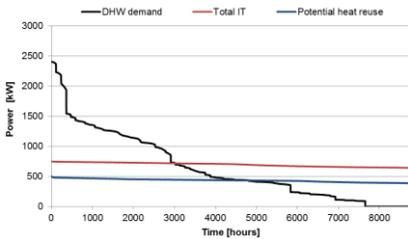
Fig. 6 Duration curve for 2,500 buildings DHW power demand and the data centre heating power generation.
