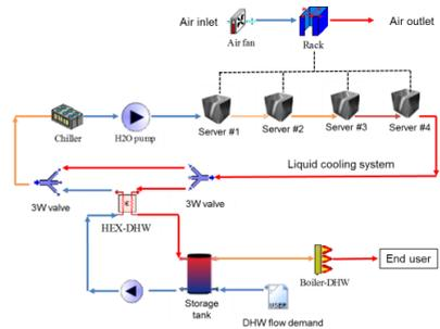
Fig. 5 Scheme diagram of the TRNSYS model for the heat reuse application.
