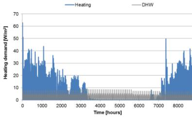
Fig. 2 Annual heating and DHW demand for a typical refurbished flat in Barcelona.
