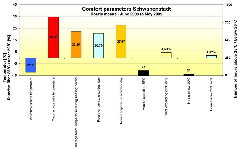
Fig. 3 Measured comfort parameters of the Secondary School Schwanenstadt during school operation from 8 a.m. to 5 p.m. (Source: AEE INTEC [3])
