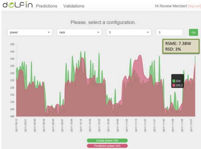
Fig. 7 Actual power demand vs forecast by the Prediction Engine in DOLFIN eCOP.
