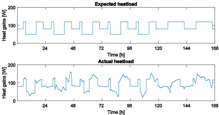
Fig. 2 Top: Expected heat load based on 24-hour static schedules. Bottom: Actual heat load, i.e. noise added to the static profile using the developed noise generator.
