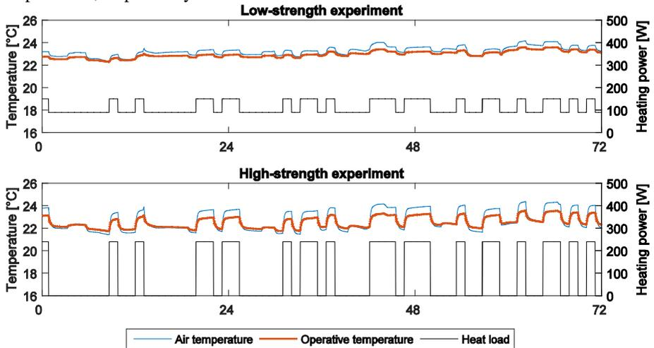
Fig. 4 Comparison of low- and high-strength experiments. Top: PRBS1, Bottom: PRBS4.
