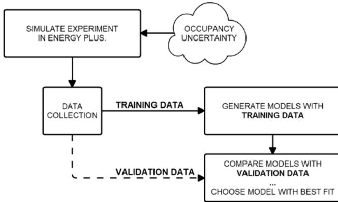
Fig. 3. System identification methodology (Hold-out cross-validation).
