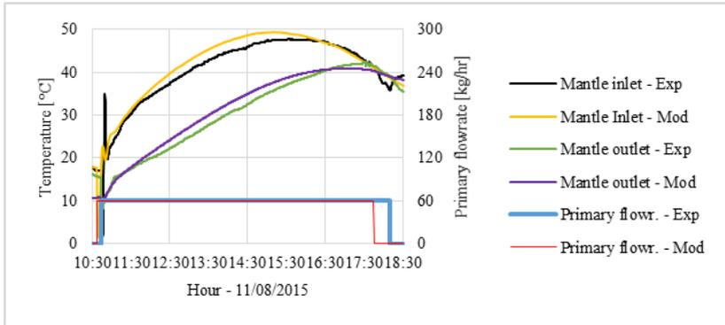
Fig. 9. Simulated and measured mantle inlet and outlet temperature and pumping period.
