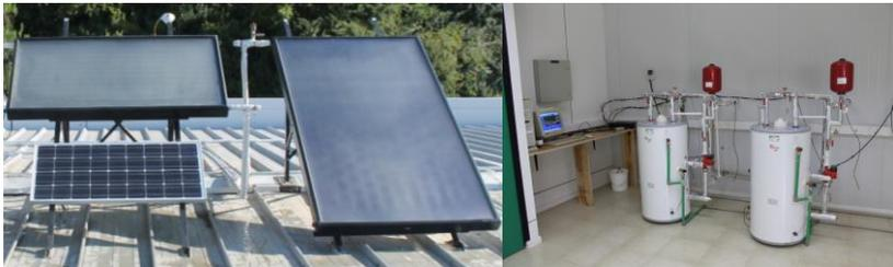
Fig. 1. Left: PV-T (upper left) and flat plate (right) collectors evaluated at the test bench. Right: Indoor experimental rig.
