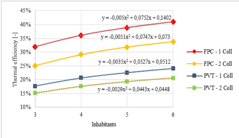
Fig. 11. Thermal system efficiency depending on the number of inhabitants and collectors.
