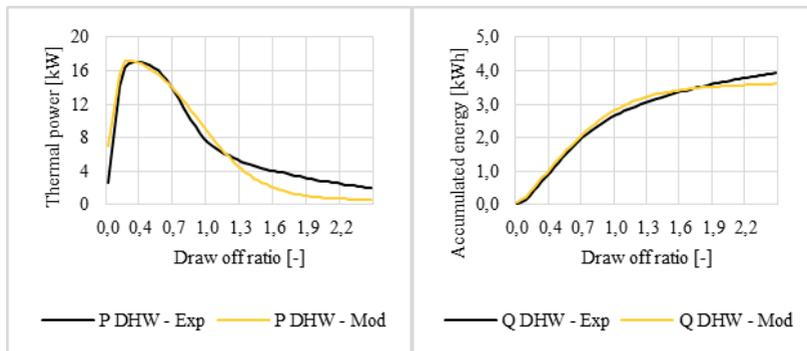
Fig. 7. Modelled and experimental thermal power and accumulated energy in the draw off.
