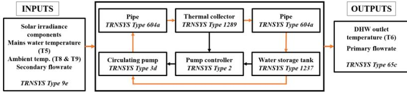
Fig. 8. Flow diagram for the entire system model validation.
