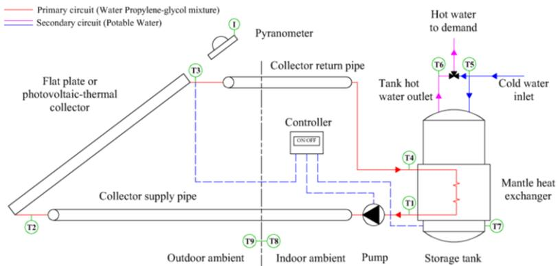
Fig. 2. Schematic diagram of the solar water heating systems in the test bench.
