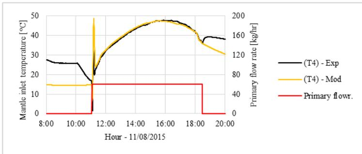
Fig. 5. Measured and modelled inlet mantle temperature for the FP collector validation.
