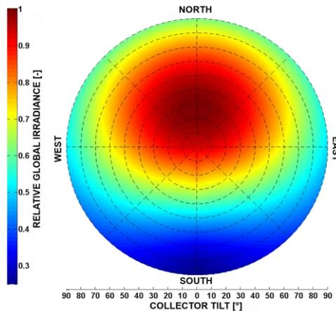
Fig. 10. Relative global irradiance on a surface depending on its tilt and azimuth.
