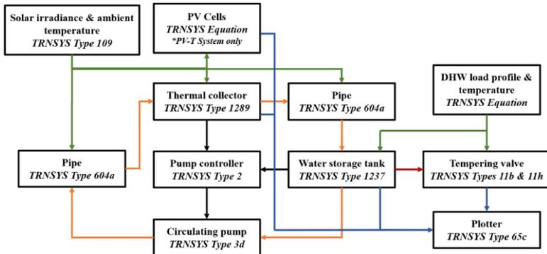
Fig. 3. TRNSYS model flow diagram for both systems.
