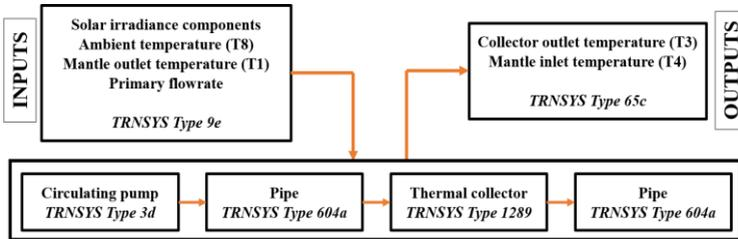
Fig. 4. Flow diagram for collector and pipes models validation.
