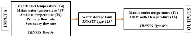
Fig. 6. Flow diagram for the storage tank model validation.
