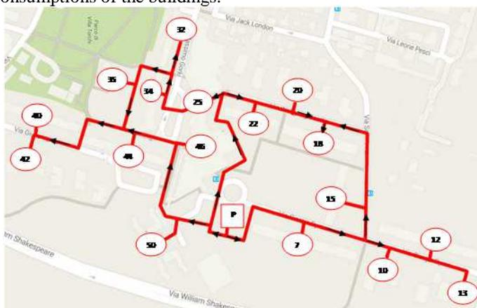
Fig. 1 Scheme of the DHS: supply scheme, gas boiler heat plant, substations
