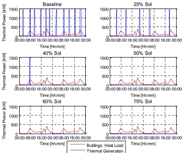
Fig. 3 Buildings' heat load and thermal output of the gas boiler for different layouts during two summer days
