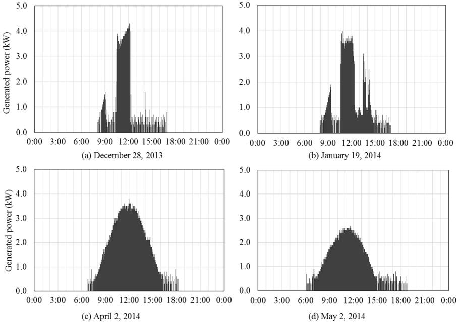
Fig. 8 Generated power after construction of adjacent buildings
