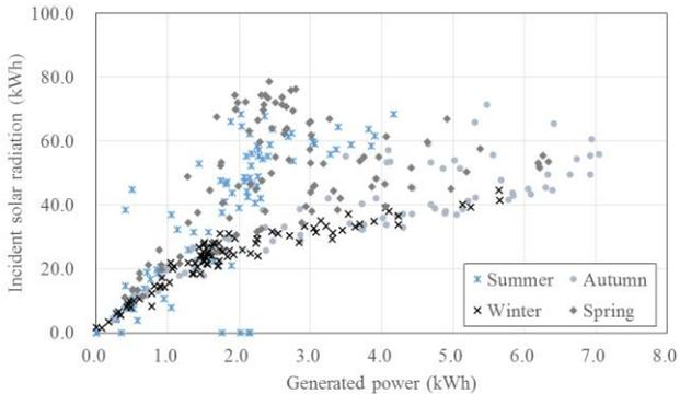
Fig. 5 Relationship between generated power and incident solar radiation
