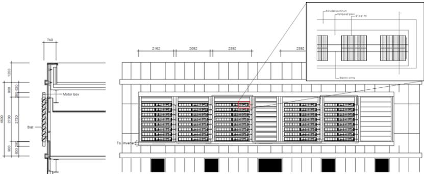
Fig. 2 Section and enlarged elevation of the lower-type BIPV
