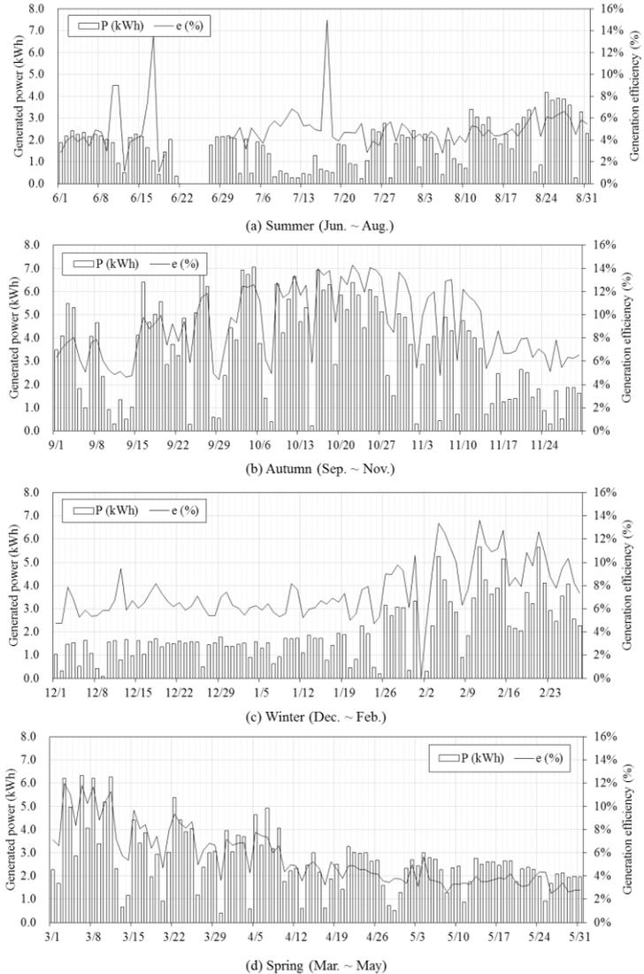
Fig. 3 Daily generated power and corresponding efficiency
