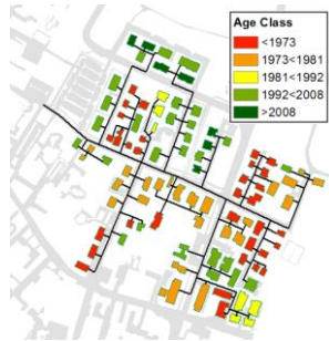
Fig. 1 Residential neighbourhood in Abano Terme with district heating network.
