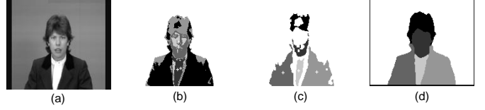
Figure 4. (a) Original image ‘Claire’, (b) Result of the KMC algorithm (Step 2, first iteration). (c) Result of the component labeling algorithm (Step 3). (d) The final segmentation after only four iterations.
