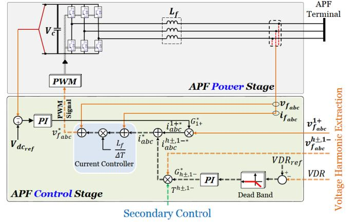
Fig. 4. APF power stage and control structure.
