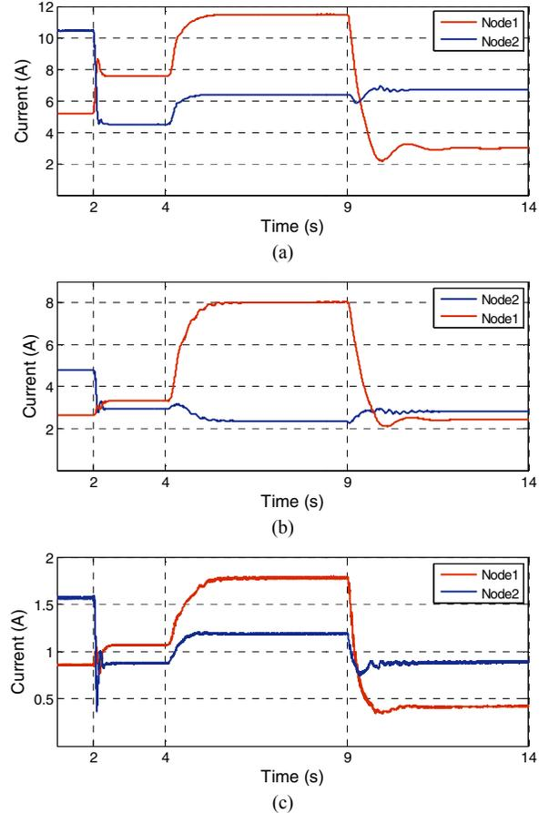
Fig. 8. Current distortion rate of nodes (RMS value in  $\alpha\beta$ -frame): (a) Fundamental negative sequence, (b) 3<sup>th</sup> harmonic, (c) 5<sup>th</sup> harmonic.
