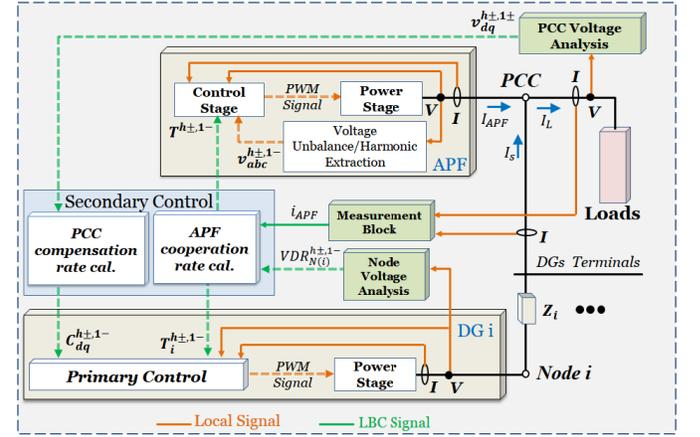
Fig. 2. General scheme of the proposed hierarchical control.
