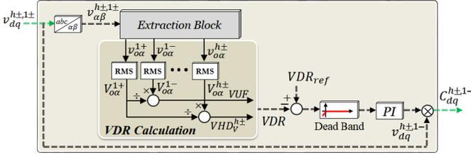
Fig. 3. Block diagram of compensation rate calculation.
