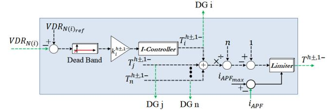
Fig. 5. Block diagram of APF cooperation rate calculation.
