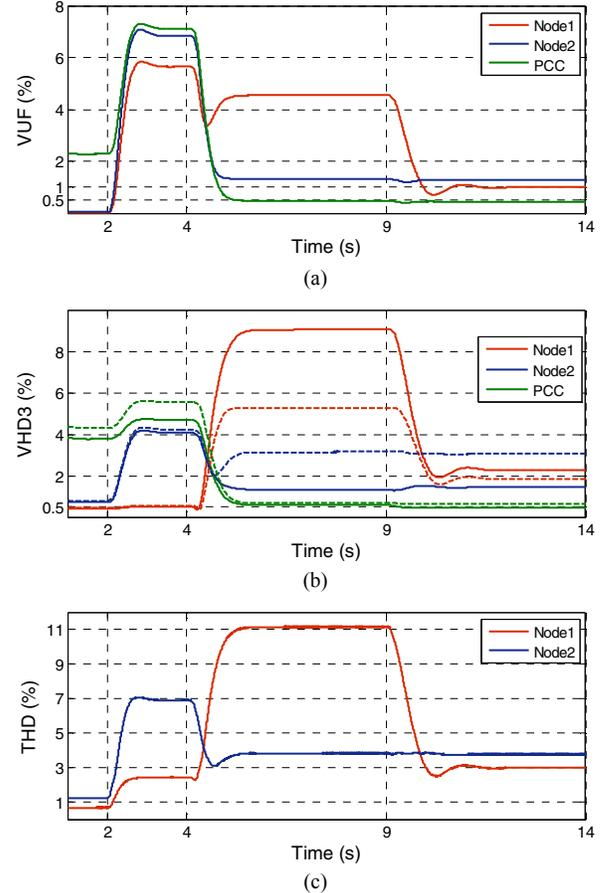
Fig. 10. Voltage Distortion Rate (dashed: positive sequence, solid: negative sequence): (a) VUF, (b) 3<sup>th</sup> harmonic, (c) THD.
