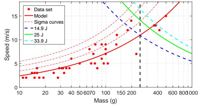
**Figure 1.** Mass versus top speed for the drone in the data set. The solid red curve is the power model, and the three dashed red curves are the  $1\sigma$ ,  $2\sigma$ , and  $3\sigma$  curves. The three joule curves at 14.9 J, 25 J, and 33.9 J are also shown.
