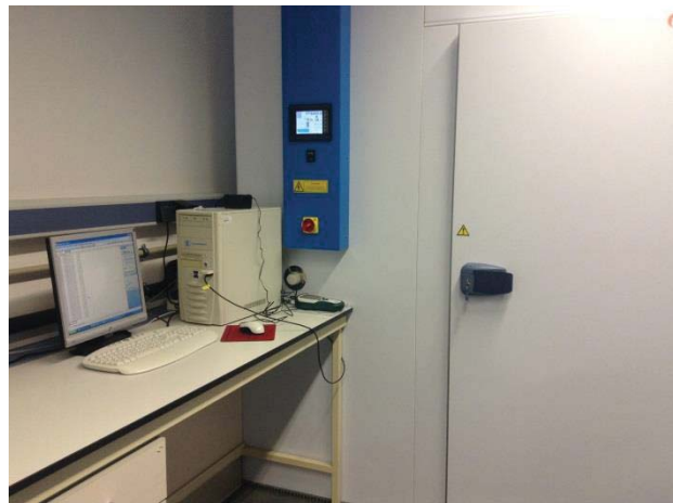
Fig. 1 Climatic chamber and data caption and register.
