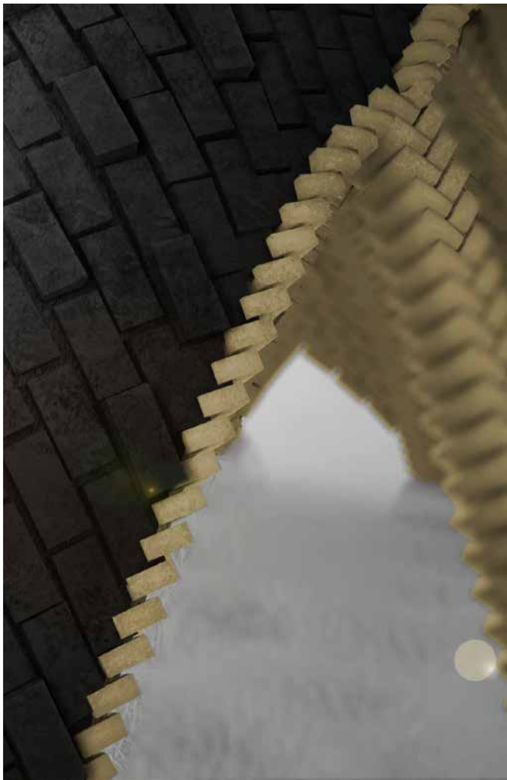
Figure 6: Rendering of pavillon assembly with outer layer of vaults in dark brick and inner vault layer and arches in light brick.
