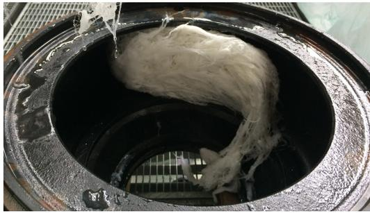
Figure 4: Clogging in the cavity after operating the pump at a part load of 60% of the BEP.
