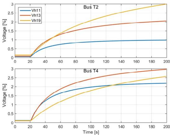
**Fig. 8.** Harmonic compensator with adaptive gain. 11<sup>th</sup>, 13<sup>th</sup> and 19<sup>th</sup> harmonic voltage levels at  $T_2$  and  $T_4$ .
