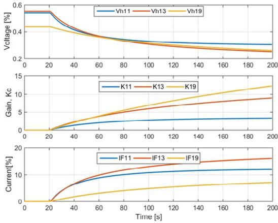
**Fig. 7.** Harmonic compensator with adaptive gain (a) 11<sup>th</sup>, 13<sup>th</sup> and 19<sup>th</sup> Harmonic voltage levels at T1. (b) Adaptive gain  $k$  (i.e.  $-K$ ). (c) Harmonic current from the STATCOM.
