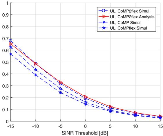
Fig. 2: UL Success Probability vs. SINR threshold.
