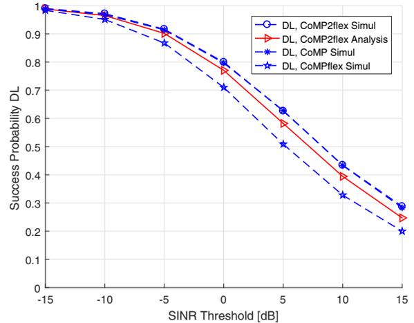
Fig. 3: DL Success Probability vs. SINR threshold.
