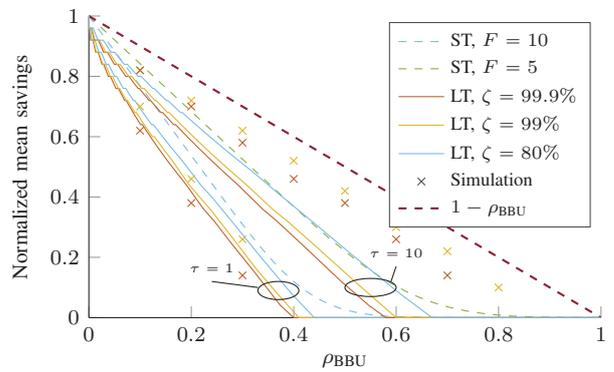
Fig. 6. Long-term (LT) and short-term (ST) server-hour savings for different mean arrival rates (reflected in  $\rho_{\text{BBU}}$ ) and  $\zeta$ -percentile queuing times.  $1 - \rho_{\text{BBU}}$  for the case with  $c = 50$  provides an upper bound on the savings. The simulation results correspond to the 99- and 99.9-percentile cases.
