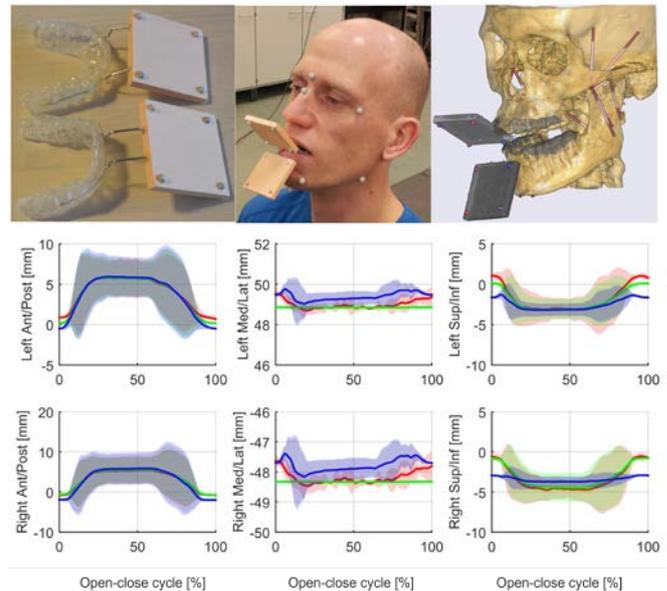
**Figure 1:** Top row from left to right: the subject-specific brace, the subject wearing the brace during the motion capture session and the musculoskeletal model driven by the measured marker trajectories of the brace. Middle and bottom rows: Predicted left (middle) and right (bottom) joint kinematics during an open-close cycle of the FDK TMJ model (blue), POP TMJ (green) and measured kinematics (red). Shaded areas indicate  $\pm 1$  standard deviation.
